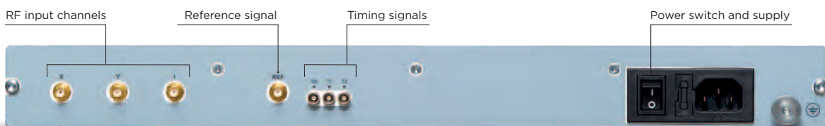
Figure 9: CavityBPM electronics based on Platform C, back panel
